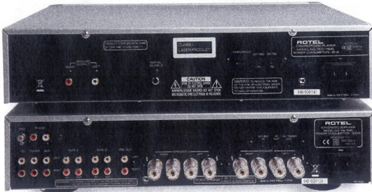
ABOVE: Single-ended analogue and digital outputs on the CD player (top) join phono, three line and two tape inputs on the amp. Switched A/B speaker sockets are fitted
